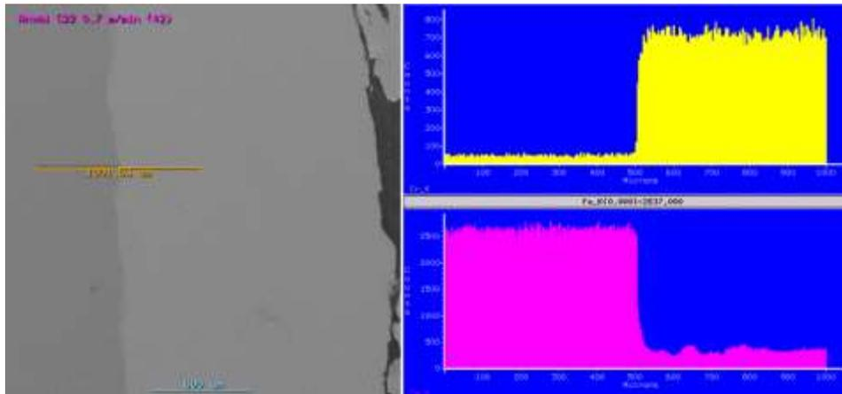
**Figure 5: NiCrMo alloy clad at 0.7 m/min, 4 kW.**
