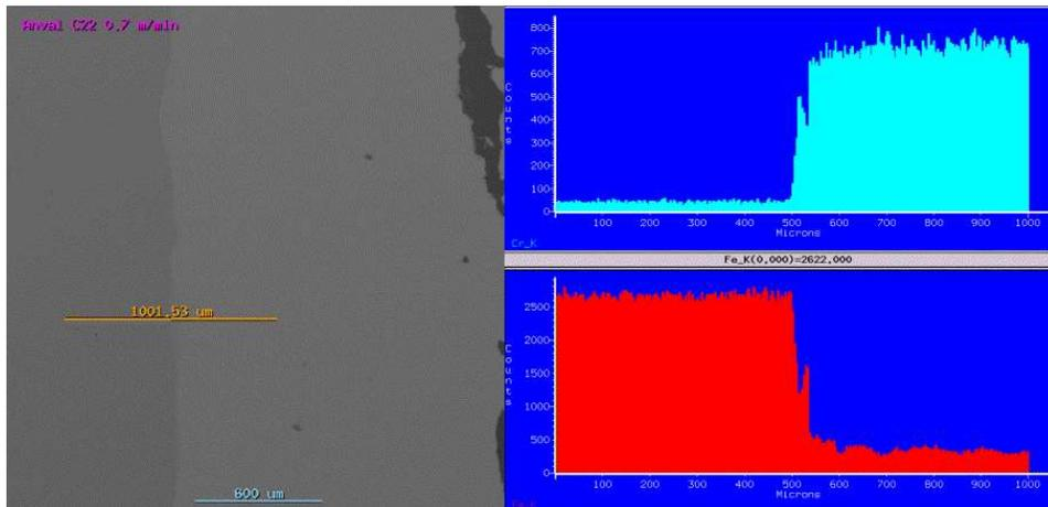
**Figure 7: SEM line trace of overlapping passes of NiCrMo alloy produced at 0.7 m/min, 4 kW.**
