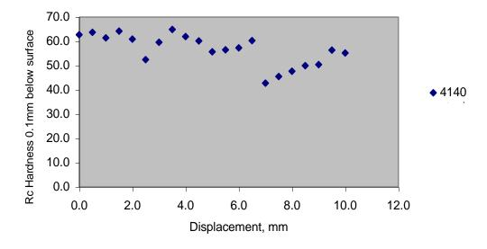
Figure 5: This figure demonstrates the effect of backtempering on hardness of a sample. The second beam was moved over 13mm after the first pass. Note, that the superhardened zone is immediately followed by the back tempered zone.
