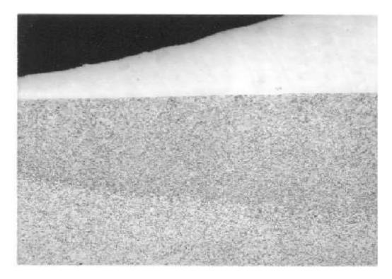
Figure 8: Inconel 625 clad taken at a magnification of 50X.
