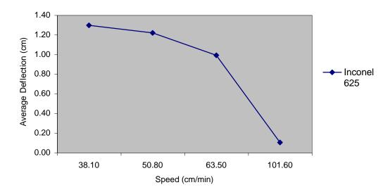
Figure 11: Average Deflection Versus speed in Inconel™625 Laser Assisted Forming.
