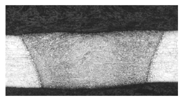
Figure 2: A Micrograph of a Stainless Steel 304 weld.
