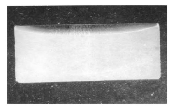
Figure 7: This photograph demonstrates the surface hardening in a 4140 steel. This picture was taken at a magnification of 6X.
