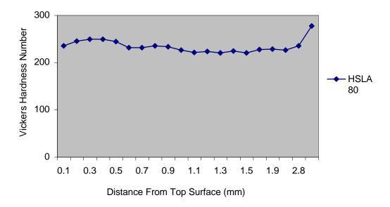
Figure 12: Vickers Hardness Number Versus Distance From Top Surface in HSLA 80 Laser Assisted Forming.
