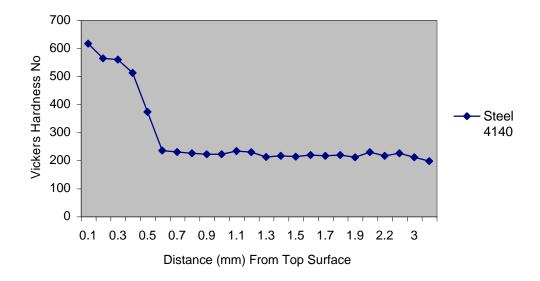
Figure 6: Vickers Hardness Number Versus Distance From Top Surface of 4140 Steel.
