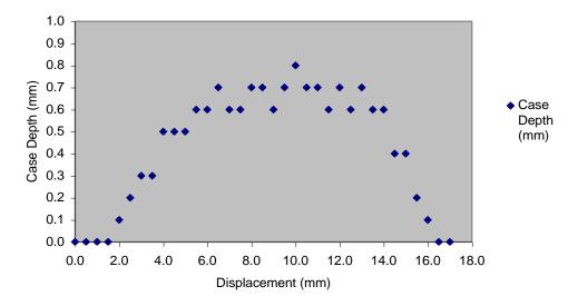
Figure 3: The hardened zone produced from a single pass, laser beam surface treatment. The beam profile is typically gaussian as shown in the above graph.
