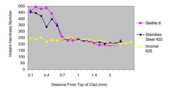
Figure 9: Vickers Hardness Number Versus Distance From Top of Clad.
