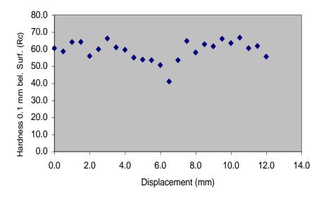
Figure 4: Superhardening has occurred in this sample as seen in the high hardness values obtained 0.1 mm below the surface.
