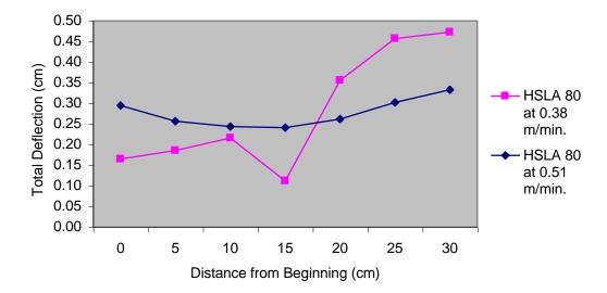
Figure 10: Comparison of Deflection Versus Distance From Beginning in HSLA 80 Steel Laser Assisted Forming.
