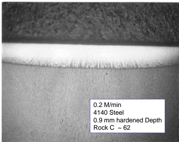
*Figure 1* – Typical profile of the hardened case resulting from a HPDDL.
