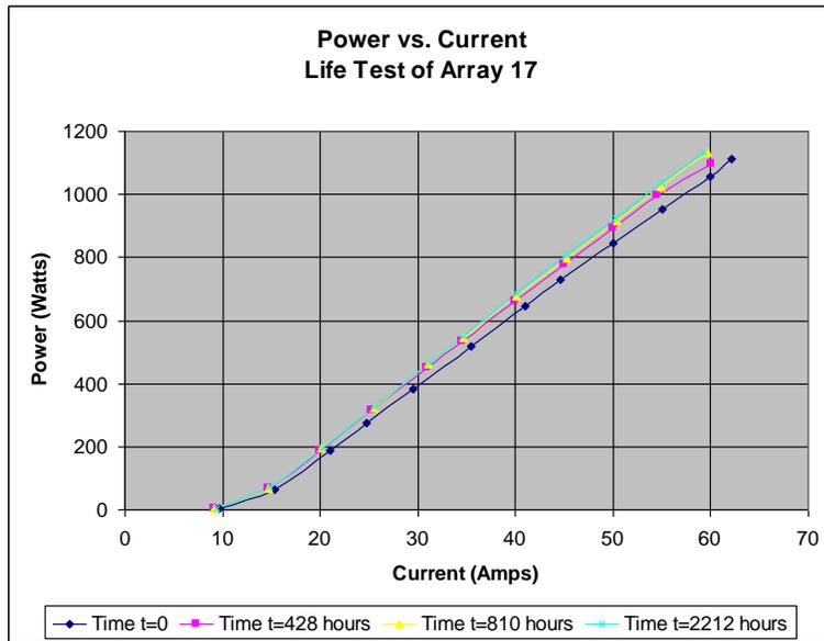
Figure 4 - After 2210 hours of pulsed operation the output power of the laser performs the same as in the CW life tests
