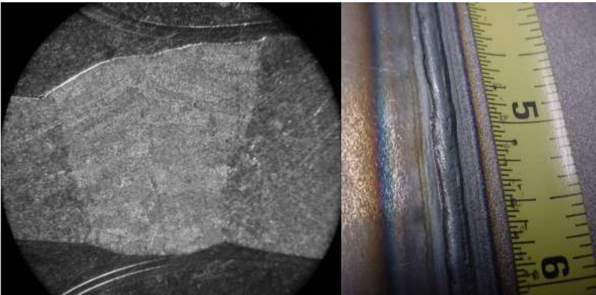
*Figure 3* - Cross section of a 3 mm – 2 mm mild steel welded with HPDDL and wire feed
