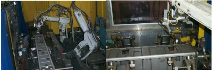
Figure 2 – HPPDL welding production installation
