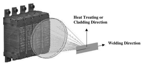
Figure 4 – Focus Configuration of Line Source HPLLD
