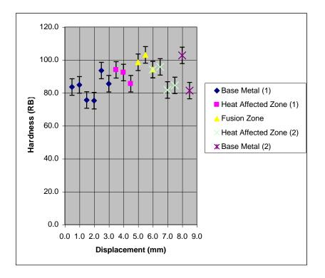
Figure 13: Hardness measurements taken across a titanium tube weld.
