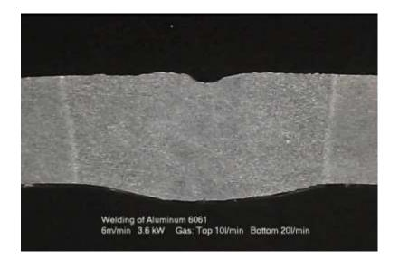
Figure 14: Micrograph of Aluminum 6061 weld at 6M/min.
