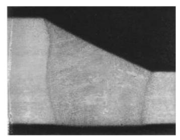
Figure 9: Micrograph of 304 SS lap weld showing excellent penetration and grain structure.
