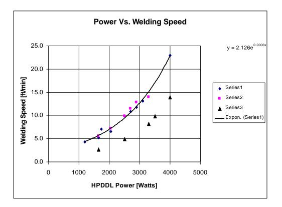
Figure 8 – Seam Welding of flat 304 SS sheets - speed vs. laser power.
