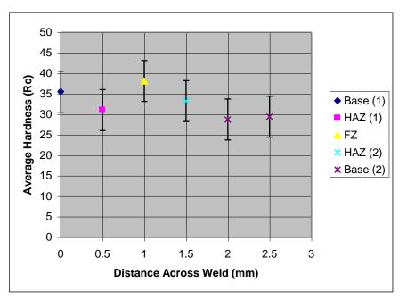
Figure 6: Average Hardness Plotted Against the Distance Across the weld for a 304 stainless steel tube.
