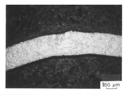
Figure 12: The fusion zone and heat affected zone of a titanium tube weld.
