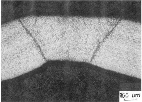
Figure 7: 304 Stainless Steel Tube Weld
